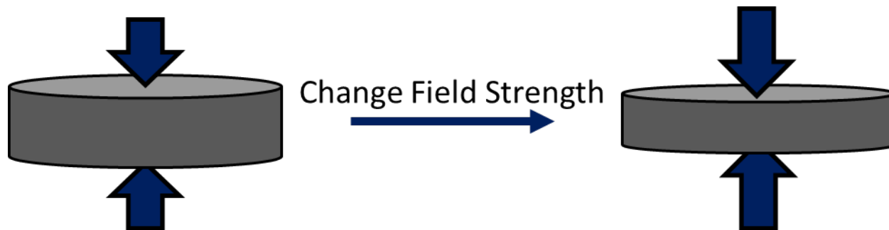
Figure: Piezoelectric ceramics are mechanically deformed when in the presence of an electric field. The reverse mechanism is also true, in that an electrical response is generated if a mechanical load is applied.
