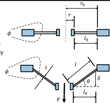
Figure 6: Membrane structure - a) Non-deformed configuration. b) Structure deformed a distance  $\delta$ . Load response,  $F$ , is measured experimentally and modeled [3]. The electrostatic potential is denoted by  $\phi$ .
