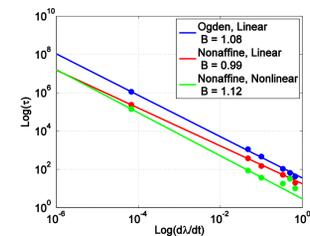
Figure 11: Power law viscoelastic behavior with respect deformation rate.
