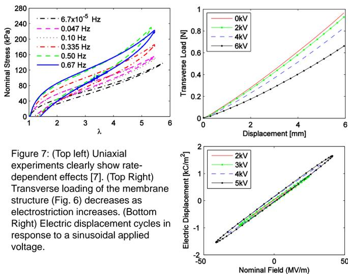
Figure 7: (Top left) Uniaxial experiments clearly show rate-dependent effects [7]. (Top Right) Transverse loading of the membrane structure (Fig. 6) decreases as electrostriction increases. (Bottom Right) Electric displacement cycles in response to a sinusoidal applied voltage.
