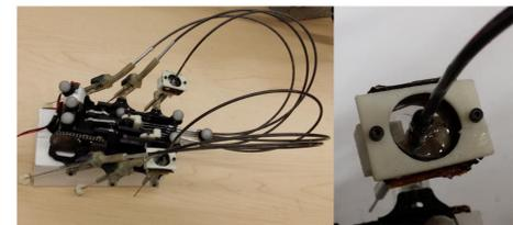
Figure 4: iSprawl robotic platform. Legs move up and down in such a way to provide forward motion.
