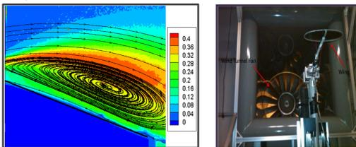
Figure 3: Wind tunnel testing of wing-shaped membrane [2].
