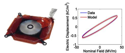
Figure 2: Model validation of electric displacement defined as a function of the nominal electric field [3].
