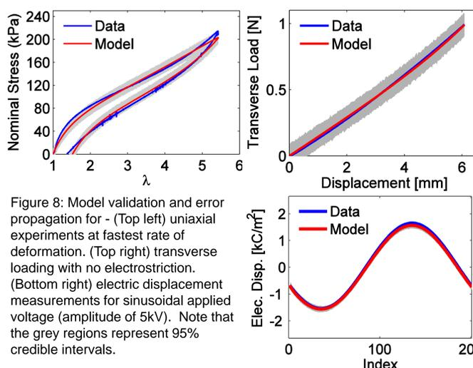
Figure 8: Model validation and error propagation for - (Top left) uniaxial experiments at fastest rate of deformation. (Top right) transverse loading with no electrostriction. (Bottom right) electric displacement measurements for sinusoidal applied voltage (amplitude of 5kV). Note that the grey regions represent 95% credible intervals.
