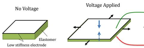
Figure 1: Activated electrodes compress, resulting in a decrease in tension and allowing for the outward expansion of the material.
