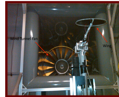
Figure: Wind tunnel experiments with deformable dielectric membrane 2 . By adjusting the membrane stiffness, the wing profile subsequently changed its shape and altered the flow characteristics.
